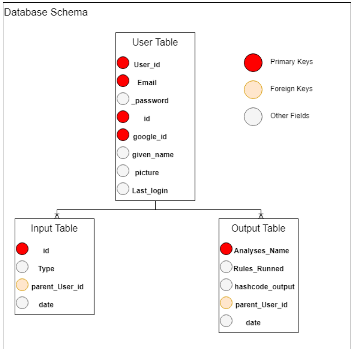
Figure 10: Database Schema with all fields and respective father and child relationships tables, containing the information about primary and foreign keys.
