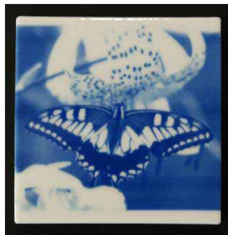
Fig. 7. (Color online) Photograph of a tile decorated by an ink-jet printing system with aqueous synthesized pigment ink.
