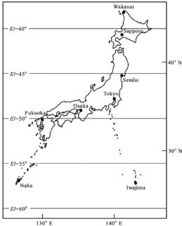
Fig.1. Japan map: elevation angle of beam direction
