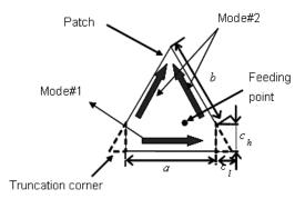
Fig.3 The two orthogonal mode and truncation corner [30]
