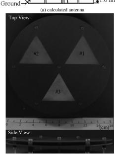
(b) fabricated antenna Fig.2. Configurations of array antenna
