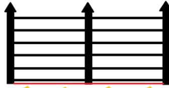
Electric wires present at ground level (under 20cm approx.)
