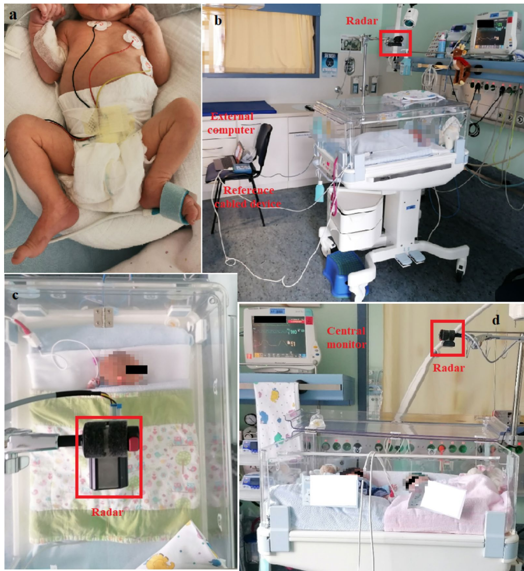
Figure 2. Clinical setup. (a) Conventional monitoring of premature neonate: connection by cables to the central monitoring unit (heart rate, oxygen saturation, respiration), and an additional peripheral venous catheter. (b) NICU room view. Both radar and the reference cabled device were controlled from the external computer. (c) Close top view. The radar was attached to a low-vibration tripod, 45 cm away from the infant. (d) Close side view with twins sharing the same bed.
