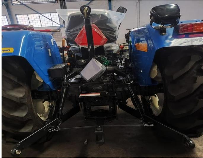
Gambar 12 Uji Coba *Three-Point Hitch*
