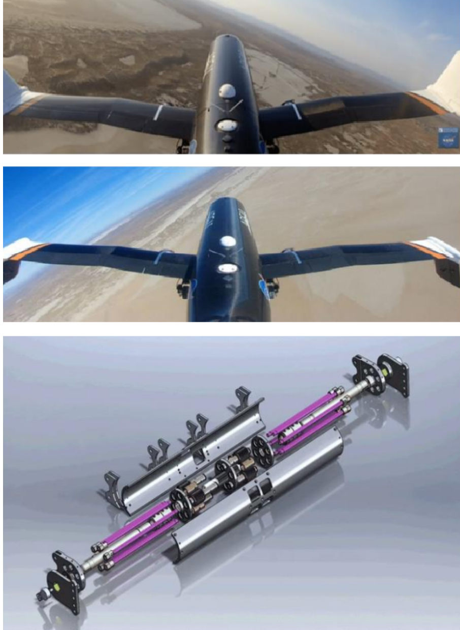
Figure 5.1 F18's folding wings and torque tube assembly for actuating the folding wings [154]
