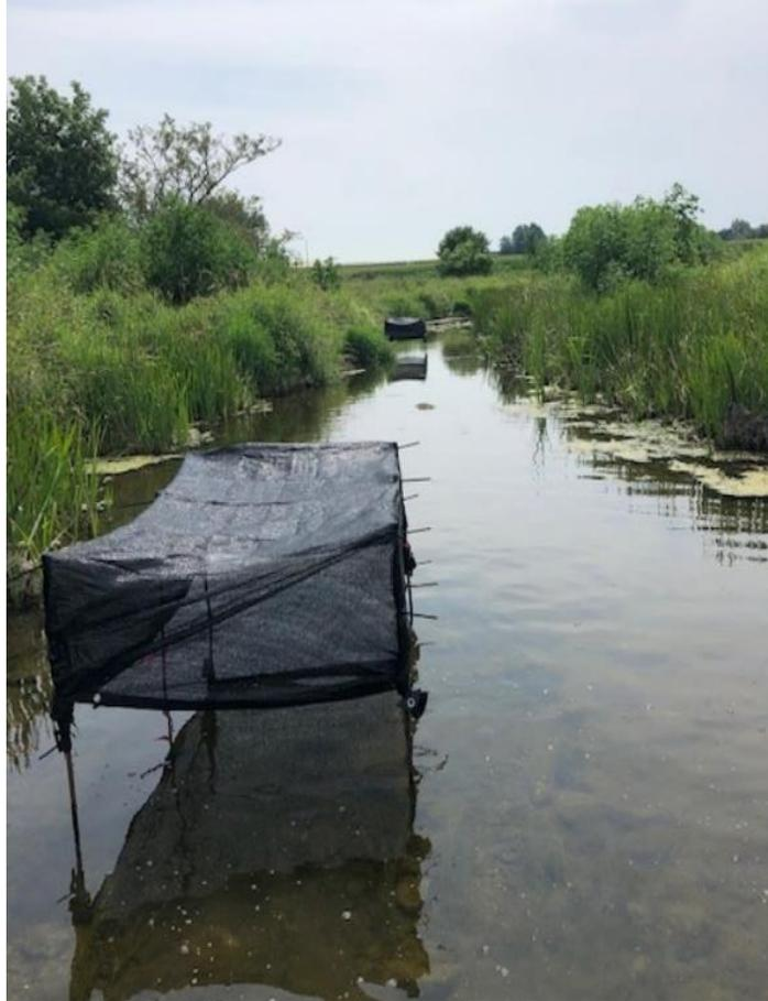
**Figure 3.4.** Experimental set-up of shaded (left) and non-shaded structures (right; located underwater) used in the field experiment conducted in southwestern Ontario, Canada. Shaded and non-shaded structures were replicated 3 times in each Moorefield Creek and South Thames River, for a total of 12 (N=12) treatment groups.
