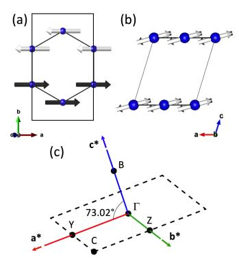
FIG. 1. The magnetic structure of NiPS<sub>3</sub> [5], viewed along the (a)  $c^*$  axis, and (b) b axis, respectively. The figure was created using the VESTA software package [7]. (c) the Brillouin zone for the magnetic structure of NiPS<sub>3</sub>. Selected high-symmetry points are indicated, corresponding to the magnetic space group  $P_C 2_1/m$  (No. 11.57) as defined in the Bilbao Crystallographic Library [8–10].
