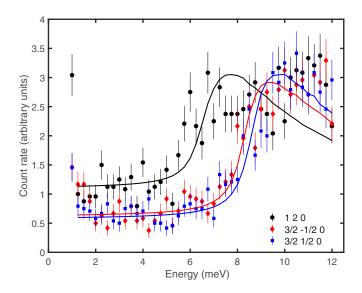
FIG. 2. Neutron three-axis spectroscopy data measured using Taipan at  $\mathbf{Q}=120$ ,  $\mathbf{Q}=\frac{3}{2}\frac{\bar{1}}{2}0$ , and  $\mathbf{Q}=\frac{3}{2}\frac{1}{2}0$ . Corresponding fits to the data are also shown and are discussed in the text.
