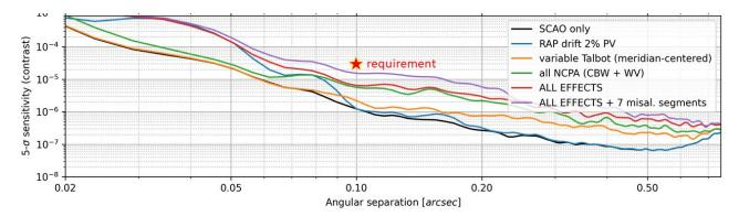
Figure 9 5- $\sigma$  Contrast curves for METIS coronagraphy with the RAVC at 3.5  $\mu$ m for a number of cases. The best case – no perturbations – is indicated by the black line; the purple line includes all effects considered. The METIS contrast requirement is shown as a red star at 5  $\lambda$ /D.
