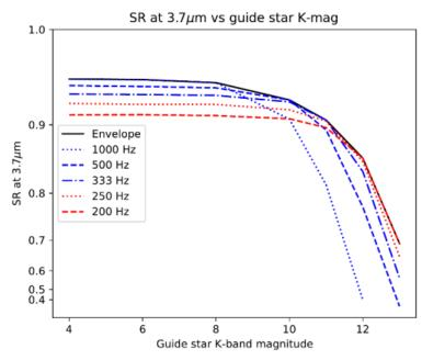
Figure 8 Performance of the METIS AO system, expressed in terms of the Strehl ratio at 3.7  $\mu$ m for a range of guide star magnitudes at K-band. For bright sources, the performance exceeds the classical diffraction limit (80% SR) by a significant margin. For fainter sources, the performance can be improved by reducing the speed of the WFS readout and thus the AO control loop [22].
