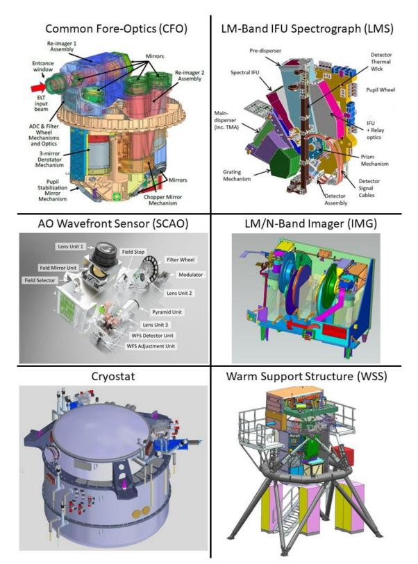
Figure 7 Opto-mechanical designs of the main subsystems of METIS (top left to bottom right): the common fore-optics, the LM-band IFU spectrograph, the SCAO wavefront sensor module, the imager, the cryostat, and the warm support structure with the warm calibration unit on top.
