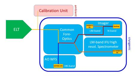
Figure 2 Simplified block diagram illustrating the conceptual setup of METIS. The colors of the beam qualitatively refer to the transmitted infrared wavelengths.
