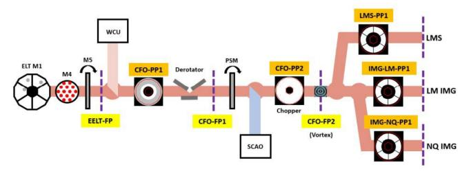
Figure 5 Schematic representation of the location of the various pupil plane (PP) and focal plane (FP) coronagraphic masks within METIS [24].
