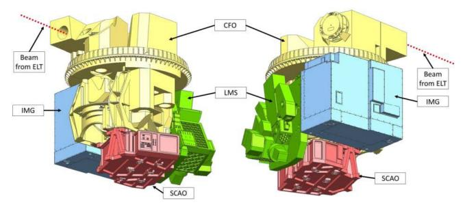
Figure 6 Two views of the mechanical design of the METIS cold optical system: the central part is the cold central structure and the common fore-optics (CFO) to which the imager (IMG) and the IFU spectrometer (LMS) are mounted. The single-conjugate adaptive optics (SCAO) wavefront sensor module is mounted at the bottom. The beam from the ELT enters horizontally near the top.
