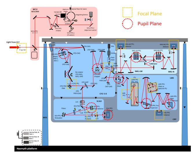
Figure 3 Functional diagram of the optical system within METIS, with a layout similar to Figure 2. All functional optical components are represented here; the beam is reduced to the optical axis. The main intermediate focal and pupil planes are indicated by yellow squares and red circles, respectively. (We note that both the LMS and the SCAO subsystem possess additional pupil and focal planes, which are not indicated here for better visibility).
