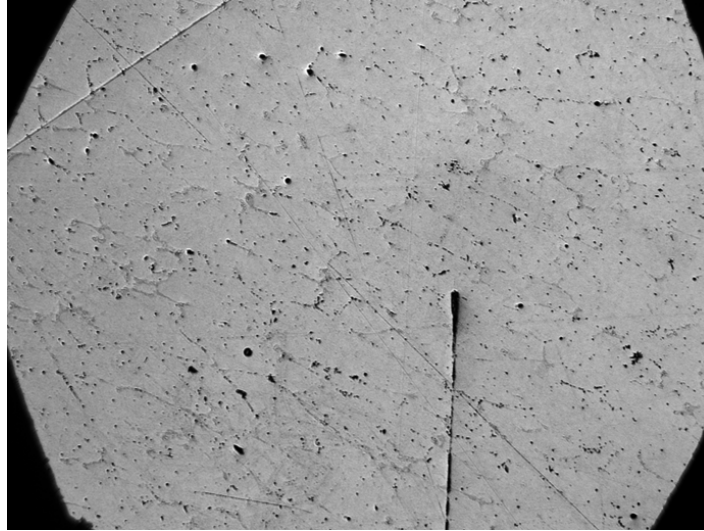
Figure 3. Normasky image obtained with the electron microscope and 5X magnification. The holes are due to the detachment of the aggregates.
