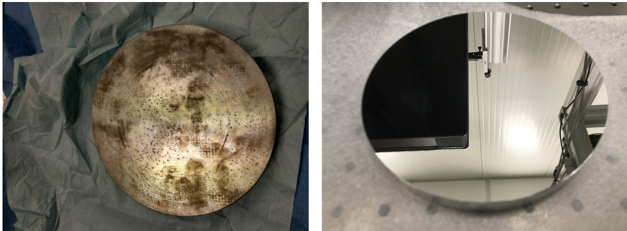
Figure 5. At left, disks with limescale deposit marks, footprints, and grid marks; at right, same disks after the Final machining and Diamond turning process, removing 0.5mm of excess metal.
