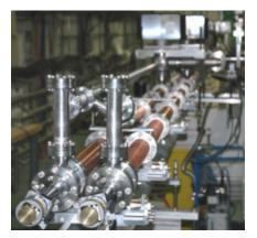
Figure 5.53.: 30 GHz SLED2 pulse-compressor in CTF3.
