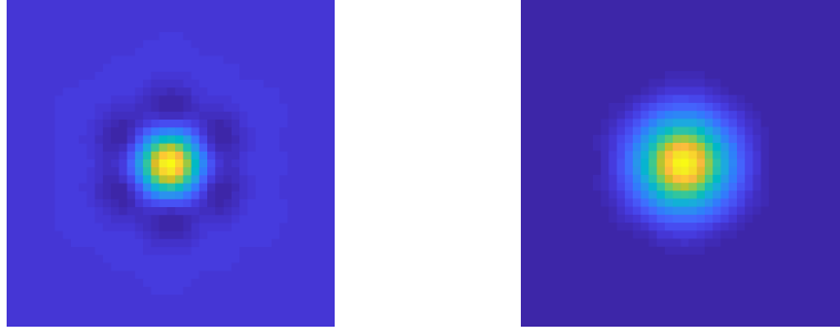
Figure 7. Example influence functions used in HARMONI SCAO simulations. Two examples are shown, the M4 influence function (left) and a 40% coupled influence function.
