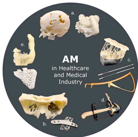
Fig. 25. Uses of AM in the healthcare and medical industry: (a) medical models; (b) implants; (c) tools, instruments, and parts for medical devices; (d) medical aids, supportive guides, splints, and prostheses; (e) bio-manufacturing [303].
