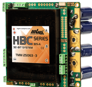
Figura 2.14 ESC HBC series V7 25063-3 de MGM-ComPro [20] .
