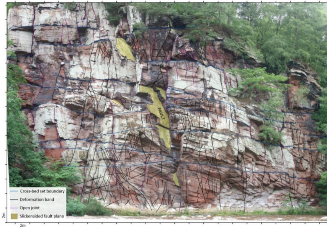
Figure 0.1: Photograph showing the distribution of deformation bands at Chain Cliff outcrop, Eden Gorge, where they are clustered around a fault plane [yellow colouration]. Deformation bands are shown in black, open joints in purple and aeolian bedding surfaces in blue (courtesy of Andrew Newell).
