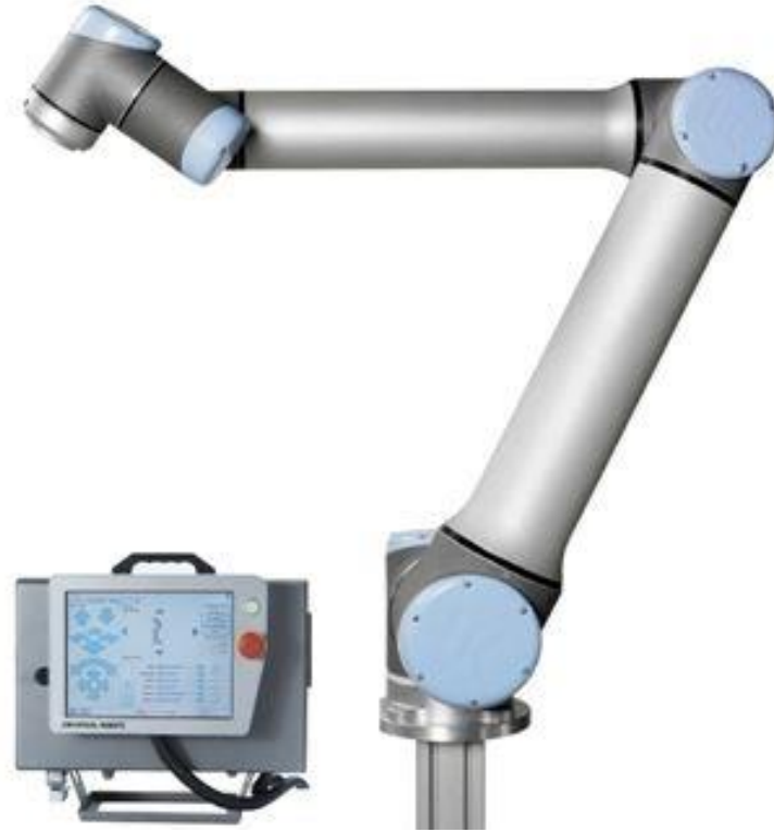
Figure 6.2-3 The UR-10 robot used in the three-dimensional localisation test. The UR robots are widely applied to industrial manufacturing. The robot system consists of a robot arm, a power module and a teach pendant. Operational programs are compiled in the teach pendant with the URScript Programming Language
