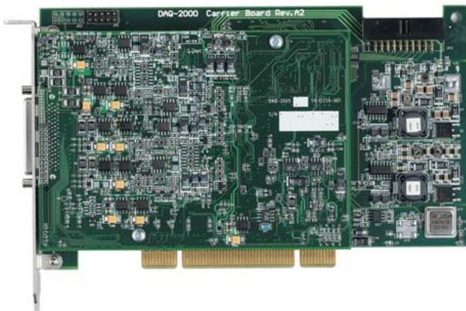
Figure 5.2-8 The DAQ-2010 data acquisition card. Parameters and functionalities such as voltage trigger, sampling rate, and pointer are adjustable through API, making it a perfect tool for particular scenarios that require acoustic sampling
