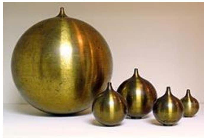
Figure 2.1-1 Helmholtz resonators. The resonators capture and amplify specific mechanical waves. The Helmholtz resonance theory was applied widely from internal-combustion engines to aircraft engines [20]
