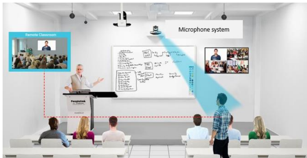
Figure 4.3-1 Illustration of the automatic acoustic tracking technology. The technology frees the speaker from holding a microphone and allows the speaker to walk freely in the space
