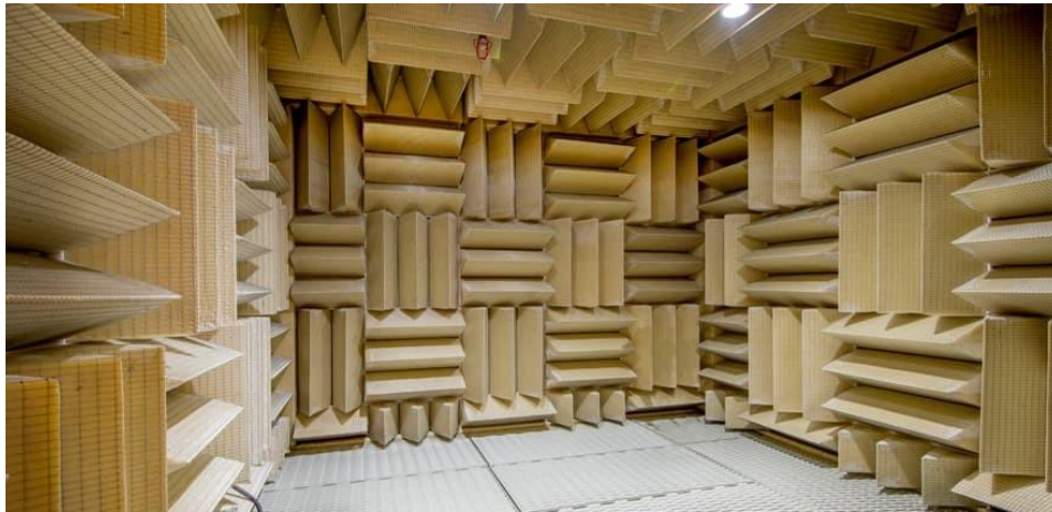
Figure 2.1-4 Sound-proof room built by Massachusetts Institute of Technology [27]. The room has a noise level of 20 dB and the wall absorbs most acoustic waves; thus, the multipath effect barely exists. The room is used for sound recording, sound quality research etc.
