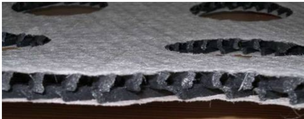
Figure 8: Cross section of FMD prototype mat showing laser cut holes to allow penetration of Permavoid ® box support struts (Puehmeier, 2009 reproduced with permission)
