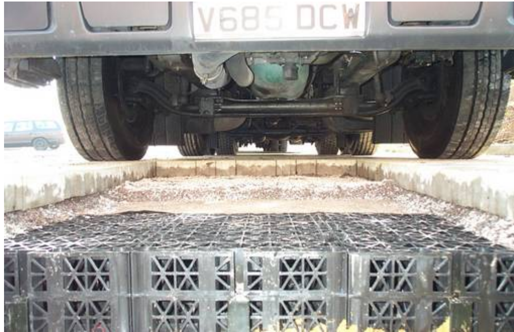
Figure 2: The candidate's Permavoid ® based experimental car park in Coventry just prior to destructive testing (Newman 2004b)
