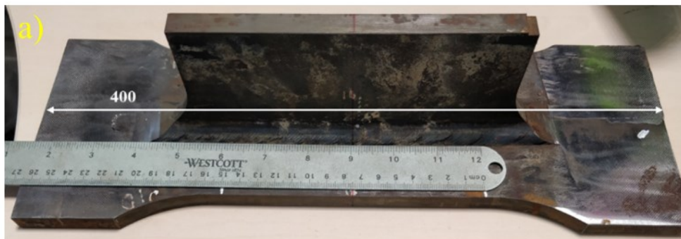
Figure 3.8: Photographs of the butt-welded plates after EDM cutting: a) Butt-welded plate with the long weld, and b) butt-welded plate with the short weld.
