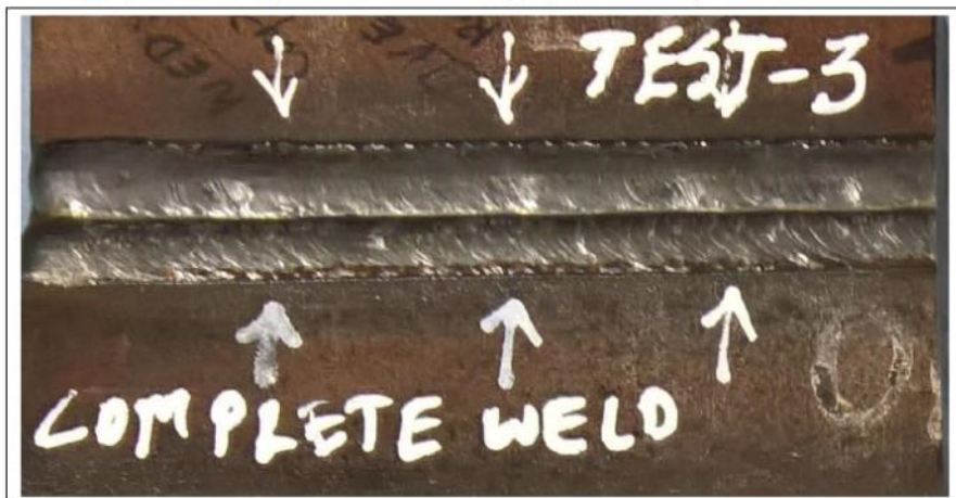
Photographs of completed weld – Radiographic identity C2453
