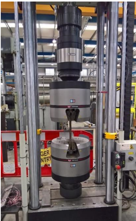
Figure 3.13: INSTRON servo-hydraulic test machine at TWI Ltd used for the application of tensile load cycles.
