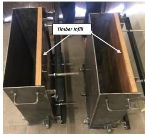
Figure 4.6: Concrete Slab Mould with Adjustable Timber In-Ply
