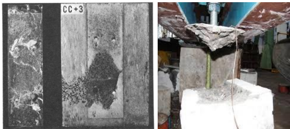
Figure 2.12: Concrete sprawling and cone failure
