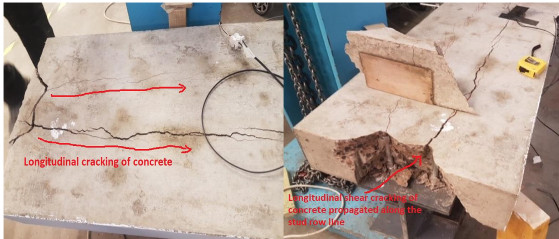
Figure 6.34: Premature failure of slab
