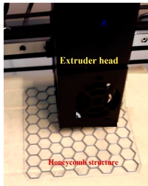
Figure 3. Layer-by-layer printing of the honeycomb structure.
