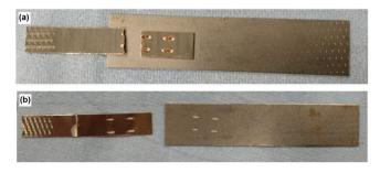
Fig. 9. The photographs of weld samples after tensile testing. (a) Laser power of 1.5 kW and failed at the HAZ of Cu. (b) Laser power of 1.0 kW and failed at the weld interface.
