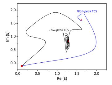
FIG. 9. Phase-space trajectories during excitation of multistable TCSs at  $\theta = -2.38$ . The initial homogeneous state is shown by a red circle and the final states belonging to *high*- and *low-peak* TCSs are marked by red crosses. Perturbation amplitudes are 1.35 and 3.9 for switching *high*- and *low-peak* TCSs, respectively, with a fixed width of 0.046 ps. Other parameter values as in Fig. 2.
