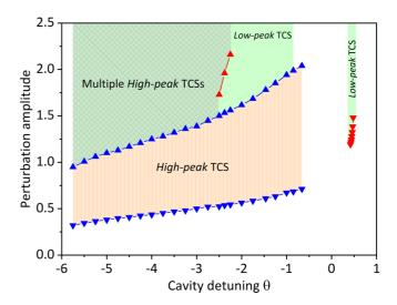
FIG. 8. Gaussian perturbation amplitude required for exciting *high*- and *low-peak* TCSs normalized to the input pump amplitude. Multiple TCSs can be excited from homogeneous solutions beyond the intermediate dynamical region (up red triangles) for  $\theta \leq -2.5$ . The width of the Gaussian perturbation is 0.046 ps. Other parameter values as in Fig. 2.
