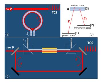
FIG. 1. (a) Schematic representation of a prototypical dispersive ring resonator device described by Eqs. (1) and (2). The black lines correspond to polarization beam splitters. (b) The  $\Lambda$  three energy level configuration. (c) Schematic representation of another dispersive resonator where the field  $E_2$  is not circulated in the cavity.
