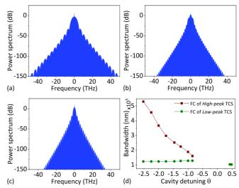
FIG. 12. Spectrum of the locked DW TCSs for (a) *high-peak* and (b) *low-peak* states of  $\theta = -2.0$ , and (c) the only TCS type (*low-peak*) of the  $\theta = +0.45$  after subtraction of the carrier frequency of the input light. (d) The bandwidth of frequency combs obtained from different types of multistable TCSs in a cavity detuning scan. FC stands for frequency comb. Other parameter values as in Fig. 2.
