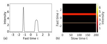
FIG. 7. (a) Intensity profile of a *high-peak* and *low-peak* TCS sequence for  $\theta = -1.5$ . (b) Slow time stability of the TCS sequence. Other parameter values as in Fig. 2.
