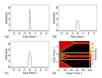
FIG. 6. Intensity profile of (a) a *high-peak* TCS and (b) a *low-peak* TCS at  $\theta = -1.5$  and (c) a *low-peak* TCS at  $\theta = +0.42$ . (d) Slow time evolution of the intensity at  $\theta = -1.8$  of a periodic pattern solution initially obtained at  $\theta = -2.3$ . Other parameter values as in Fig. 2.
