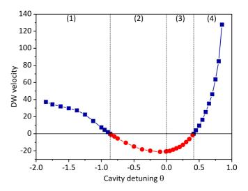
FIG. 4. Velocities of the DWs (femtoseconds/round trip time) in a cavity detuning scan. Stationary DWs at the two Maxwell points can be seen in the zero crossing of the curves. Other parameter values as in Fig. 2.
