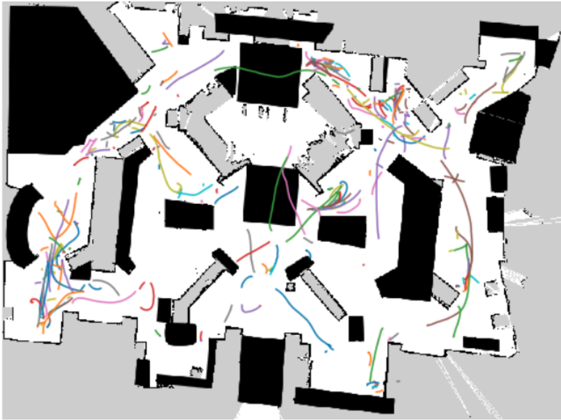
Figure 3.16: Trajectories generated by the visitors helping the robot when unable to navigate. Note most locations where human help was given are clustered in the same few areas. Black areas are no-go zones for robot navigation.
