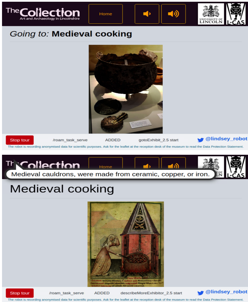
Figure 3.7: Screenshots of the graphical interface displayed by the robot’s touch screen during a guided tour. (top)During navigation toward an item location, and (bottom)during a description of the item. Any robot utterance that comes out of the speakers is replicated on the screen, as shown on the bottom image.
