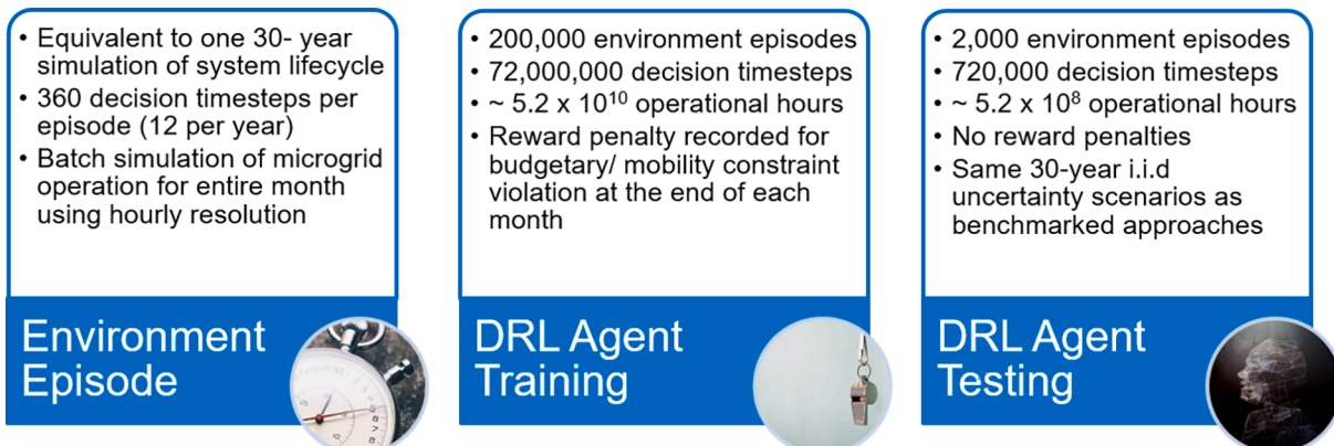
Fig. 6. Different timestep resolutions implemented for the proposed DRL approach.
