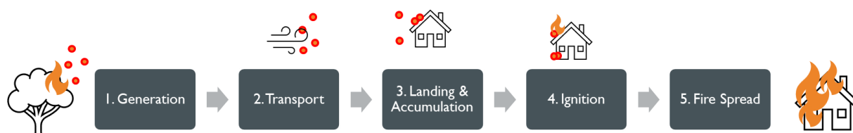
Figure 3-2: Diagram of five stages of wildfire firebrand exposure and ignition of buildings: firebrand generation, wind-driven transport, landing and accumulation, ignition and fire spread.
