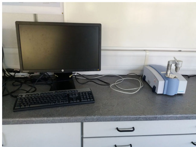
Figure 1. The Bruker Alpha FTIR spectrometer equipped with ATR diamond holder.
