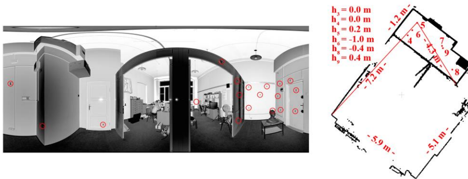
Fig. 7. The point cloud example in the spherical projection of Test Site V with marked check points (red circles) [63].
