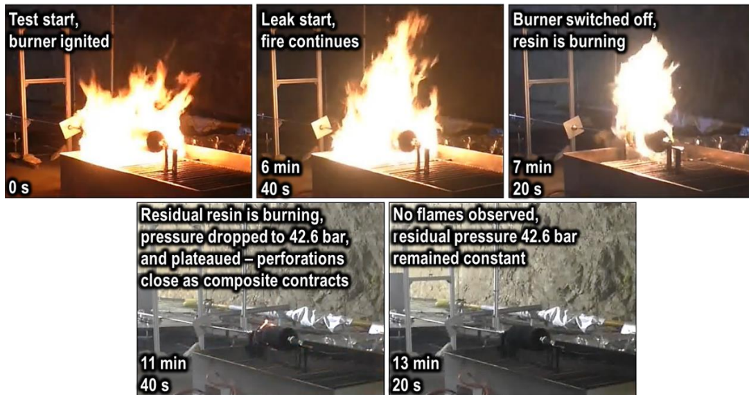
Figure 1. Snapshots of the \mu LNB tank fire test with COPV#CB-1
