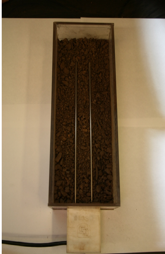
Figure 2.5 Water Content Reflectometer and constructed PVC box with substrate during calibration. An equal depth of substrate was added above the sensor prongs prior to calibration.
