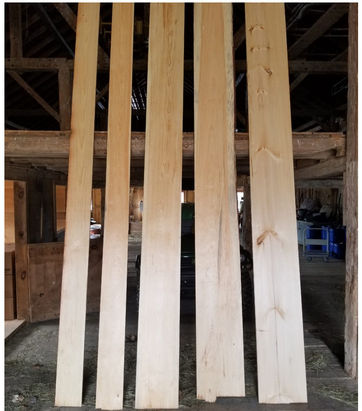
Clear lumber from pruned pines. The board on the right shows the core of the tree at the size it was pruned (Photo credit: Jim Frohn, UNH Extension)
