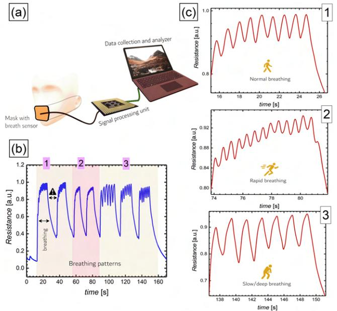
Fig. 5. (a) Schematic of the respiratory setup utilized. (b) The breathing response in real time recorded using annealed (700°C) Ge:SiNWs. (c) The data marked as 1, 2 and 3 expanded.
