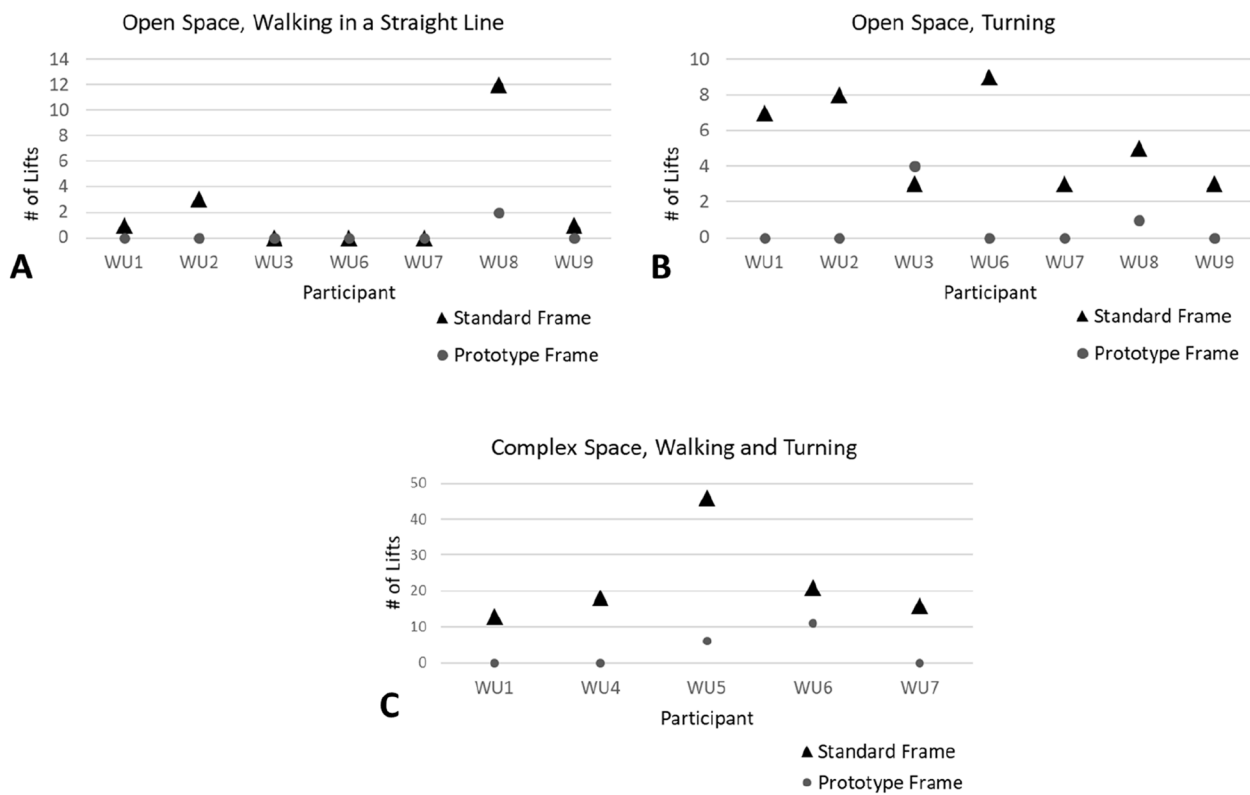
Fig. 4 Lifting events (less than 3 frame legs are grounded). Individuals’ data (WU1-WU9) for the standard frame and the prototype frame are shown for walking in a straight line in the Open Space (A), turning in the Open Space (B), and walking in combination with turning in the Complex Space (C)
