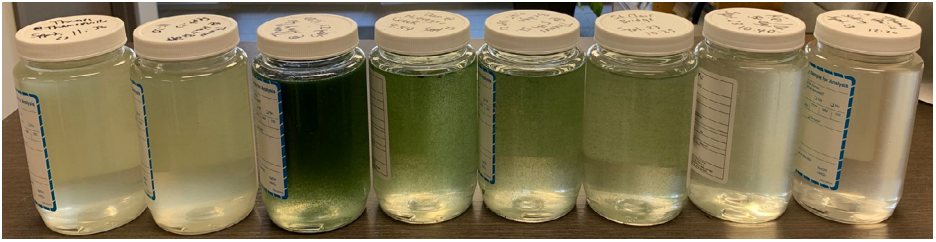
Fig. 1. Samples from near surface of Thames River acquired on September 23, 2019. Survey extended from Thamesville, ON (far left; 64 km from river mouth) to Prairie Siding, ON (far right; 14 km from river mouth). Samples in middle with distinct green discoloration were acquired from a 9 km stretch of the river through Chatham, ON.
