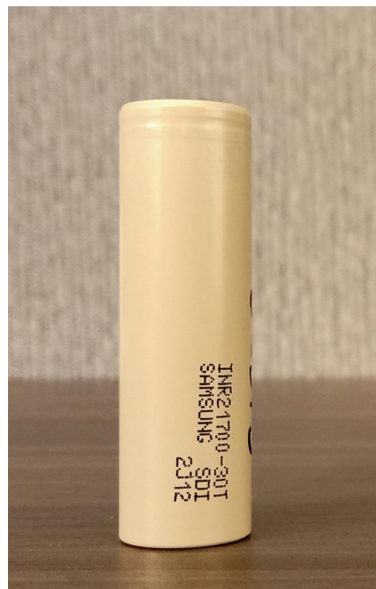
Figure 2. Samsung-30T INR21700 Li-ion battery
