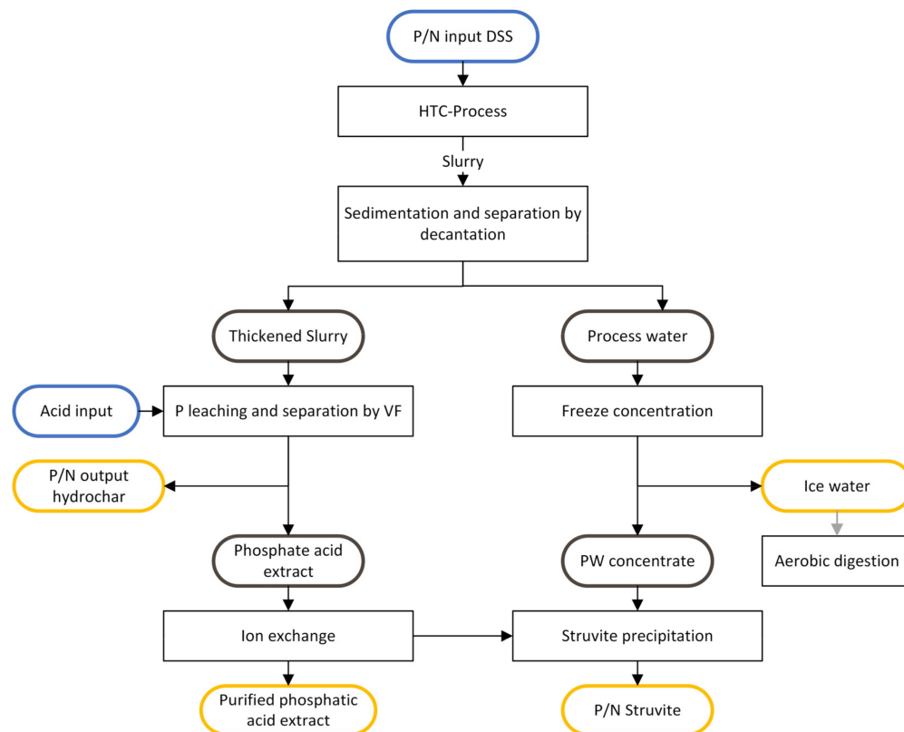
Figure 1. Flow chart of experimental setup. (P = phosphorus, N = nitrogen, DSS = digested sewage sludge, HTC = hydrothermal carbonization, VF = vacuum filtration, PW = process water).
