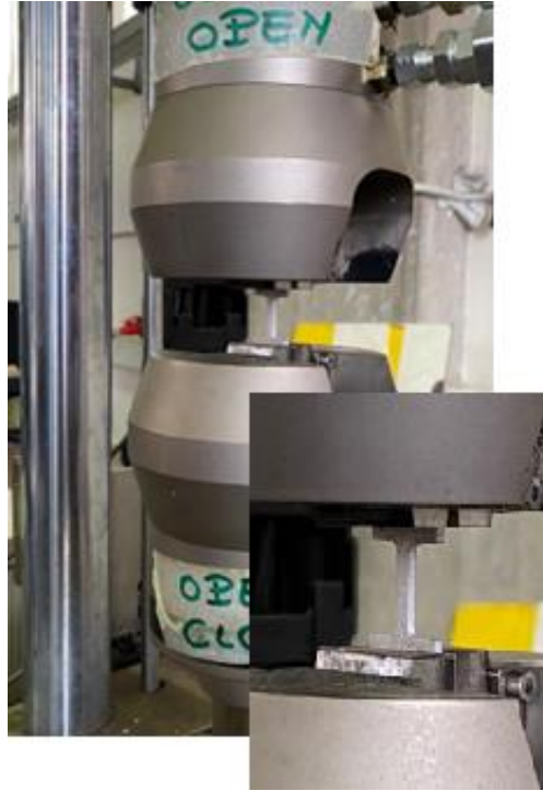
Figure 3.7 – Specimen mounting/positioning on the testing machine.
