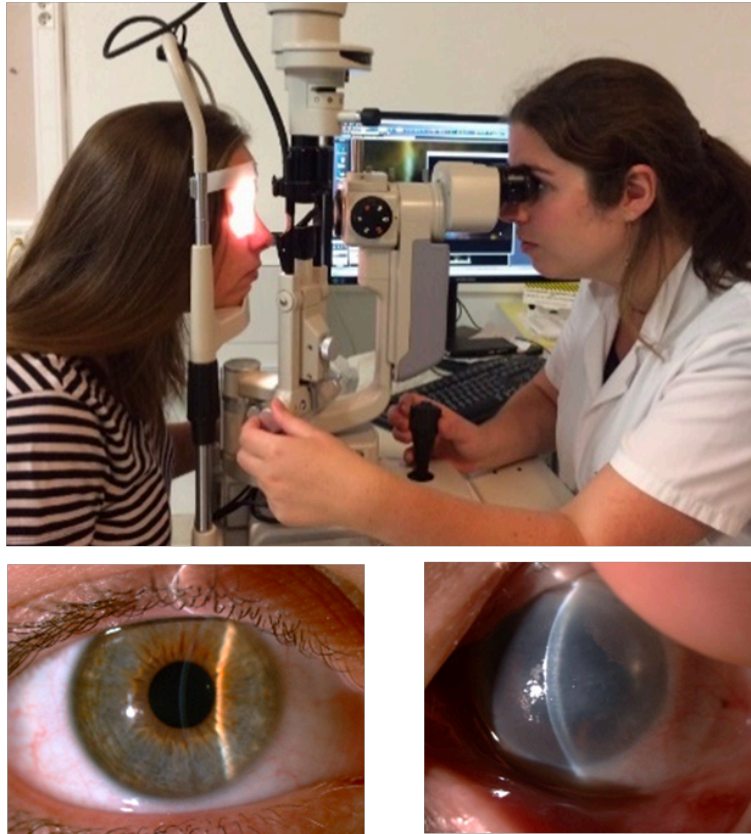
Figure 1.14: Top: Image of a slit lamp biomicroscope. Bottom: Slit lamp images of a healthy cornea with low scattering (on the left) and a pathologic cornea with high scattering (on the right). Taken from [2]
