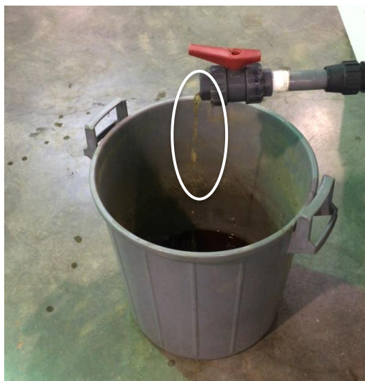
Figure 18: Example of the outflow considered in the saturation process (constant outflow during at least 10 min).
