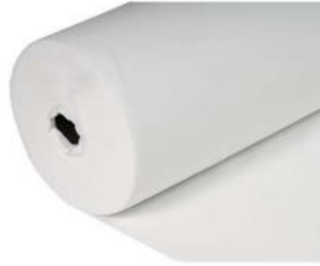
Figure 6: Nonwoven polypropylene fiber filter layer [29].
