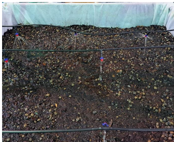
Figure 17: Sprinklers used to the precipitation simulation tests.
