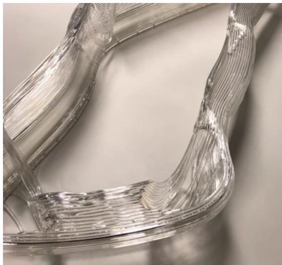
Figure 22- Organic test part with fallen layers due to the Lh being too big.
