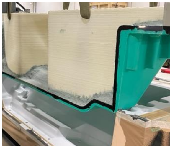
Figure 28- Support structure of a dashboard counter mold made from PP30%GF.
