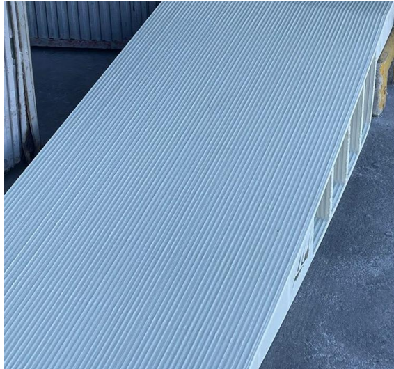
Figure 49- Periodic defect visible through the whole part.
