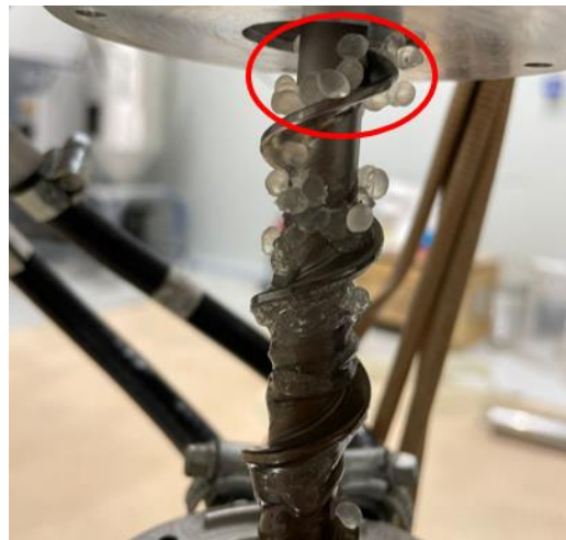
Figure 41- Pellets stuck in the extruder chamber.
