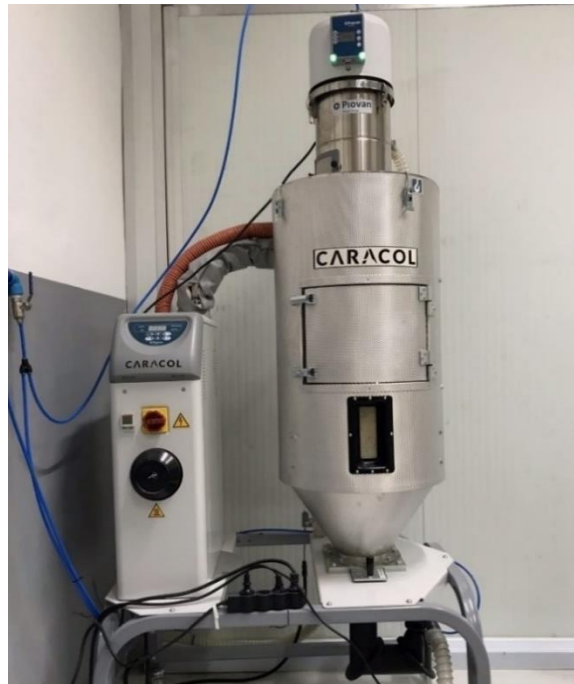
Figure 12- Dehumidifier system from Piovan.
