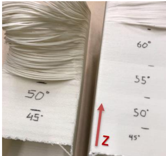
Figure 21- Test parts made with the same material, for different layer heights.
