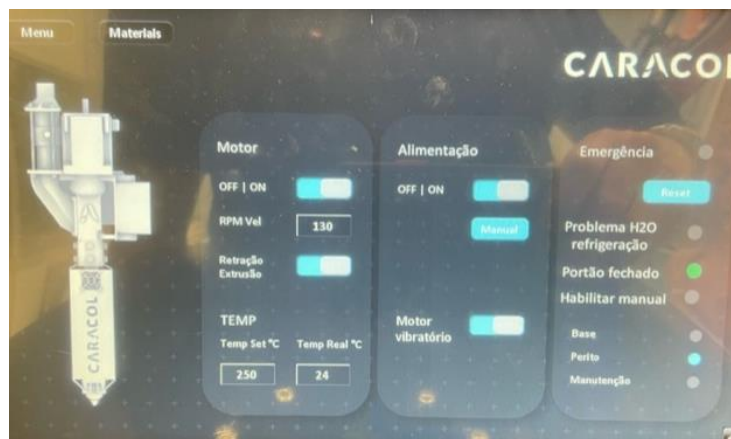
Figure 11- Controller for the extruder.
