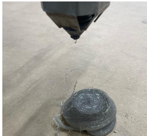
Figure 17- Purge of material.
