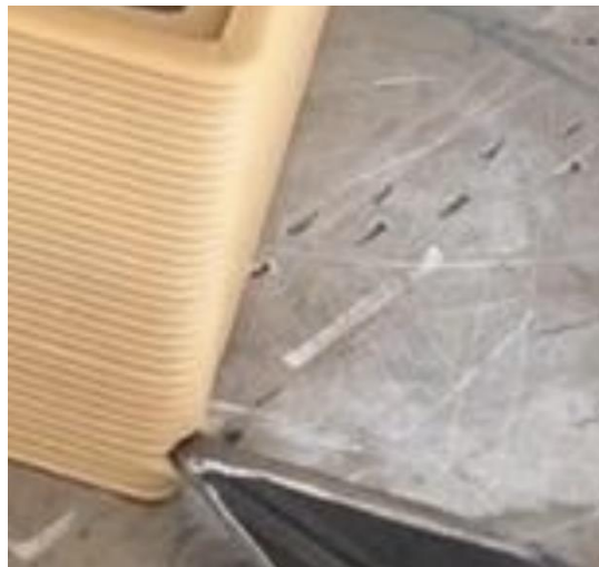
Figure 51- Mechanical fixture used to secure the parts to the construction platform [36].
