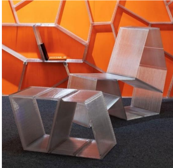
Figure 45- Furniture parts printed in PETG.
