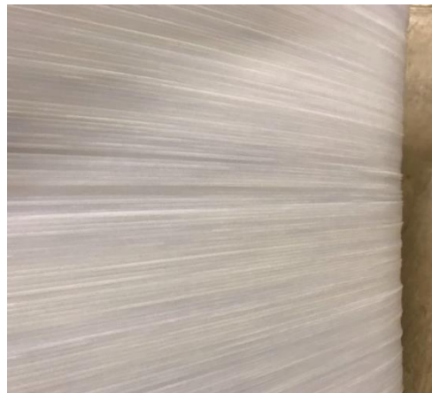
Figure 37- Color heterogeneity on the surface of a recycled PET part.
