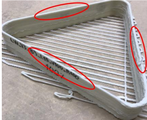
Figure 19- Part created in the experimental tests and its measurement zones.
