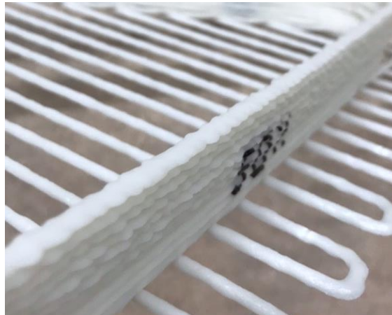
Figure 20- Example of a not acceptable surface.
