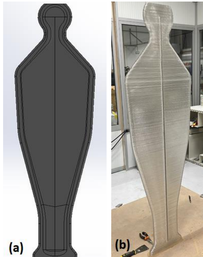
Figure 44- Final dummy created: solidworks model (a); printed part (b).
