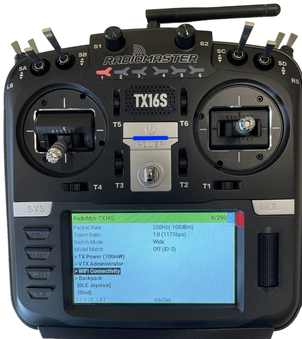
Figure 4.14: The ELRS Lua script used for configuring the ELRS module in the remote controller.
