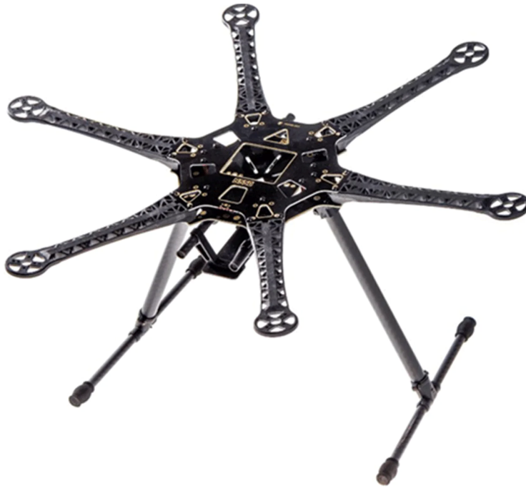
Figure 2.1: Example of a drone frame. [1]
