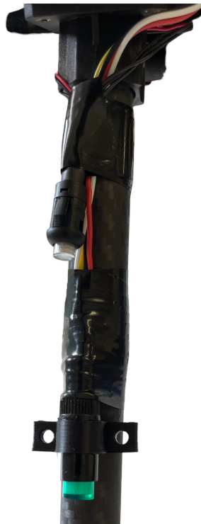
Figure 4.8: Flight controller's (top) and power distribution board's (bottom) buttons, attached to one of the frame's legs.
