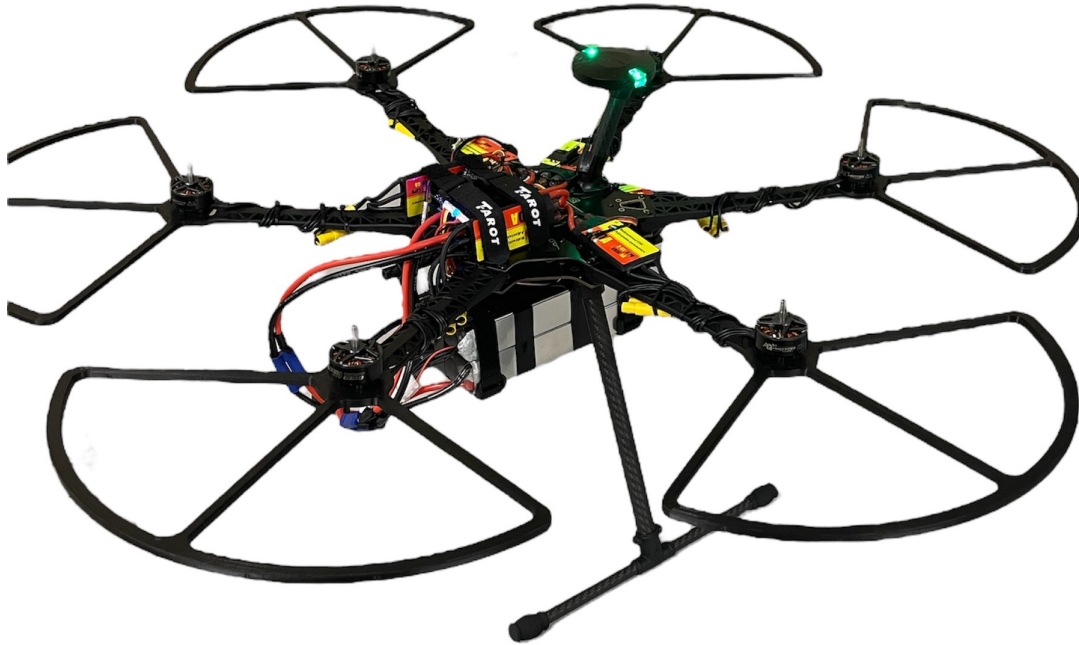
Figure 4.11: The finished, complete build, missing only the propellers.
