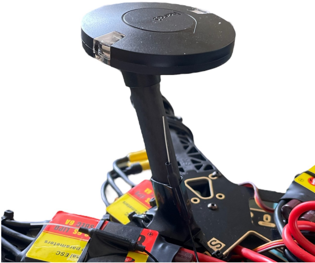
Figure 4.10: The GPS after mounting it to the frame. One of the receiver's antennas was attached to it.
