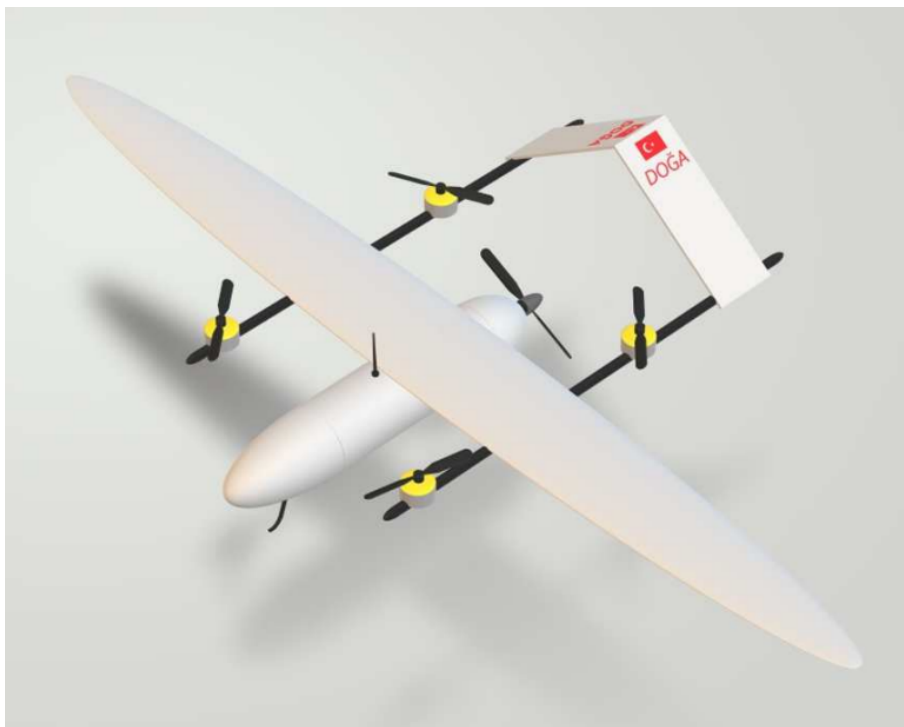
Figure 2.13: 3D rendered model of a VTOL UAV designed in [11].
