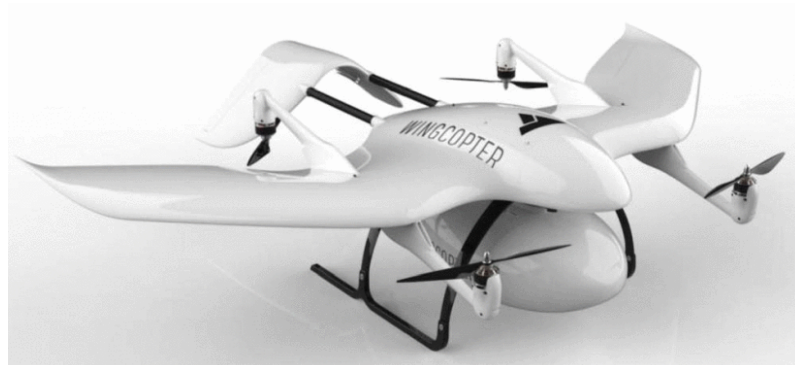
Figure 2.9: The HealthDrone is based in a widely available hybrid drone, the wingcopter 178.[8]
