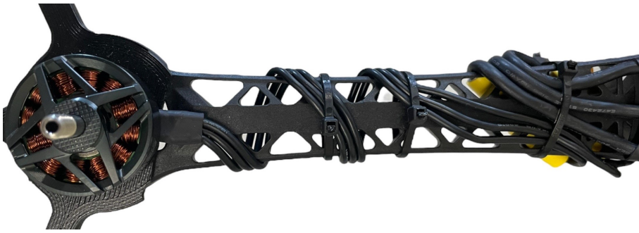
Figure 4.5: One of the arms with tidied cables.
