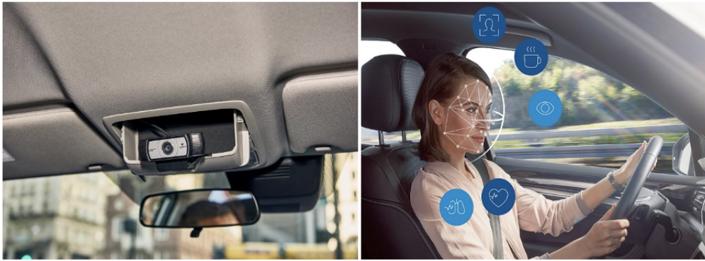
Figure 3.1: Internal video camera (on the left) and monitored signals examples captured with an internal video camera (on the right) [9].
