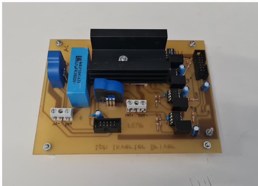
Figure 5.8: Single phase inverter with current sensors.
