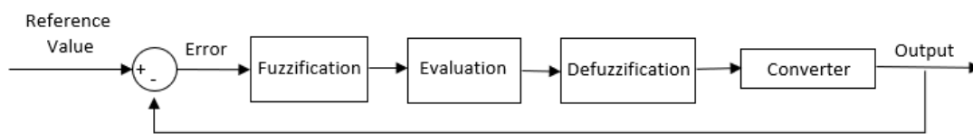
Figure 2.16: Fuzzy control feedback diagram
