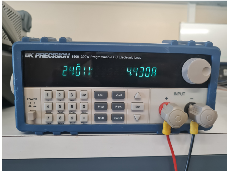
(a) Electric load values (Voltage and current input) with maximum 24 V set.
