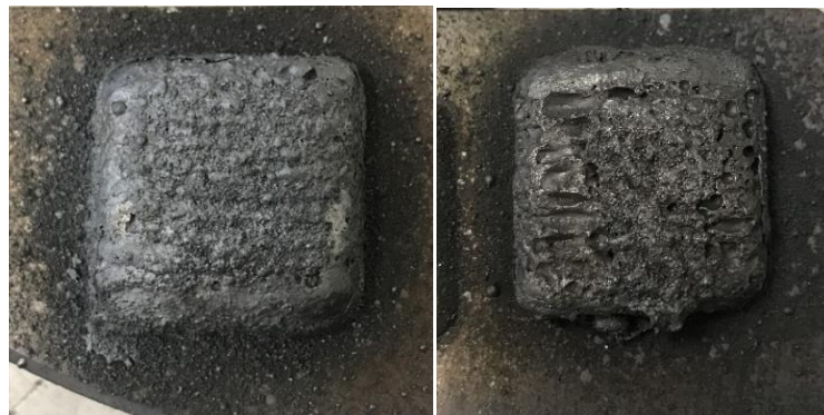
Figure 4.19 - Printed multilayered volume with the optimized parameters.
