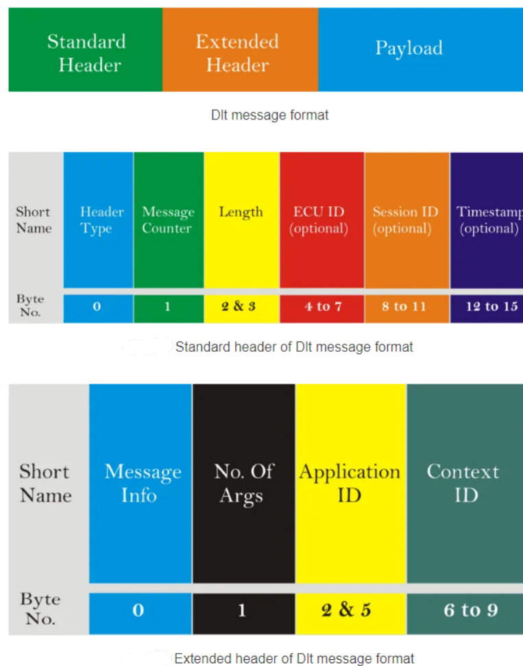
FIGURE 2.4: Message format of DLT protocol[23].
