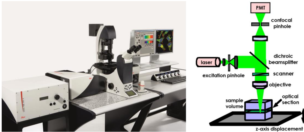
Figure 1.14 - Leica® TCS SP5 microscope setup (right) and schematic illustrating the principle of CLSM (left). PMT - photomultiplier tube. Adapted from www.leica-microsystems.com and (101).
