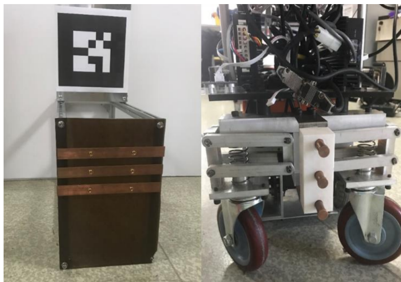
Figure 2.31: (a) The docking and charging station. (b) The robot docking mechanism robot we developed [9]
