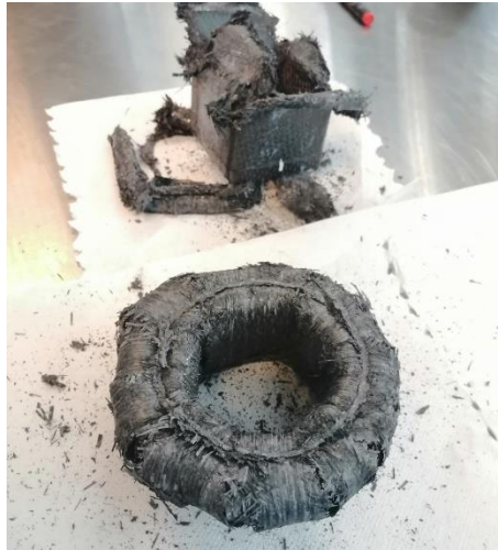
Figure 21 - Round and square tubes after crushing
