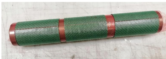
Figure 18 - Flax fibres wrapped around the mandrel
