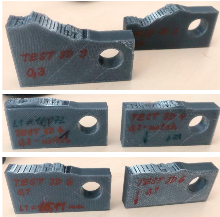
Fig. 7. Fractured CT specimens: Regular 0.3 mm (Top); SGed 0.3 mm (Middle); Regular 0.1 mm (Bottom).
