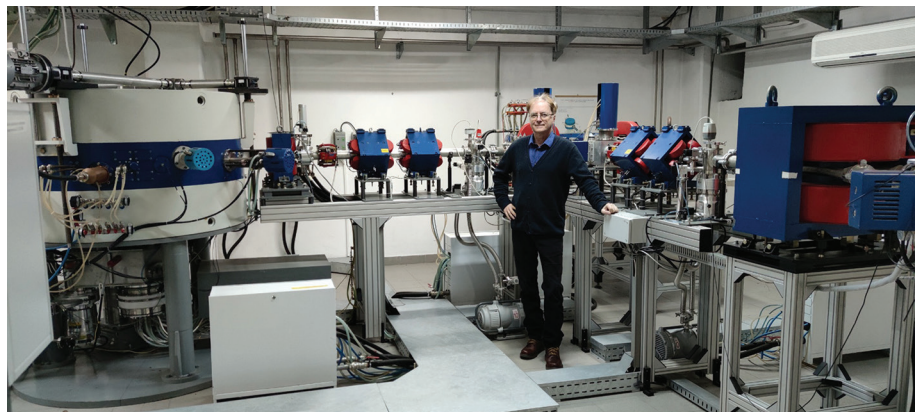
Figure 3. Upper photograph: The proton cyclotron complex (1–3 MeV, 10–100 nA) of the channels C5 and C6 for ion-beam analysis of materials of the FAMA, Institute Vinča (R. Balvanović). Lower photograph: The target area of the channel C6 for analysis in-air (in construction). The Si(Li) Detector C6-D1 is for trace elements detection, the SDD detector C6-D2 is for matrix elements, and the C6-D4 is for dose measurements. The portable gamma detector, for ultra-light matrix elements (not shown), is shared with channel C5. The samples are placed on a target holder assembly (C6-TH), equipped with x and y motors for scanning samples with proton beams.
